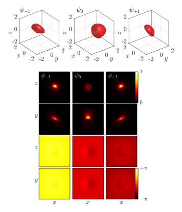
FIG. 15. Most unstable eigenfunction for the first AR solution for  $\mu = 20$ , with the same layout as in Fig. 5. The most unstable eigenvector does not carry a sizeable amount of vorticity and thus isocontours of vorticity have been omitted. Please refer to Appendices A and B2 for details on the BdG formulation and the numerical methods involved.
