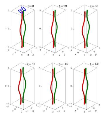
FIG. 18. Destabilization dynamics for the first AR for  $\mu = 16.5$  giving rise to a homoclinic orbit. The vortex filaments move in a cycle depicted by the blue arrows in the first panel. The layout and perturbation are the same as in Fig. 7. See Supplemental Material [53] for the corresponding movie.
